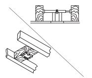
Before installing this fan make sure the outlet box is properly installed to the house structure. To reduce the risk of re, electric shock, or personal injury, mount to outlet box or supporting system acceptable for fan support. (Mounting must support at least 35 lbs.)
