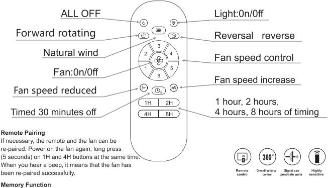
After a power outage or a tripped circuit breaker, the fan will default to Fan ON and the fan will run at the speed that was last saved in memory.
