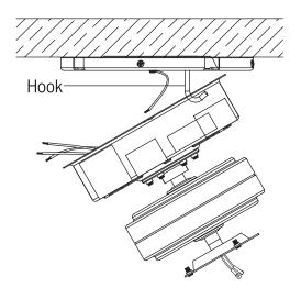
3. Mounting plate for hands-free wiring and safety cable installation.
