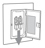
Before you begin installing the fan, Switch power off at Service panel and lock service disconnecting means to prevent power from being switched on accidentally. When the service disconnecting means cannot be locked, securely fasten a warning device, such as a tag, to the service panel.
