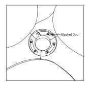
1. Install blade with screws provided , aligning each of the holes as shown and tighten all screws securely. Repeat this process for remaining blades.
