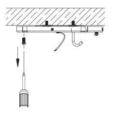
1. Loosen 2 screws across from each other and remove the other 2 preassembled screws from mounting plate (Corresponding to installation step 5). Save screws for later use.
