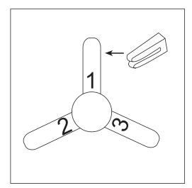
Slide the balancing clip on the trailing edge of any blade, halfway between the holder and tip. Run the fan to check the wobble. If the wobble persists, repeat with each blade, noting which one most reduced the wobble.
