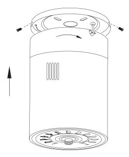
Lift motor assembly, aligning the keyhole slots with the preassembled screws on mounting plate, and twist clockwise till lock.
