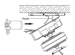
2. Once wiring step has been completed, slide the wired remote receiver in between the mounting bracket and the top plate of motor.
