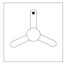
Stick the adhesive-backed balancing weight on the top center of the blade directly in line with the balancing clip.Add more weight if needed to get a smooth-running fan.
