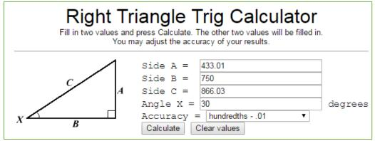
Side A = Minimum Downrod Length = 433mm - Round length up (450mm).
